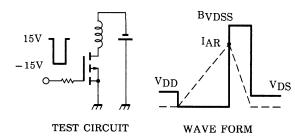
$$\begin{array}{ll} R_G \!=\! 25\Omega \\ V_{DD} \!=\! -25V, \; L \!=\! 10mH \end{array} \qquad E_{AS} \!=\! \frac{1}{2} \cdot L \cdot I^2 \cdot (\frac{B_{VDSS}}{B_{VDSS} \!-\! V_{DD}}) \end{array}$$
